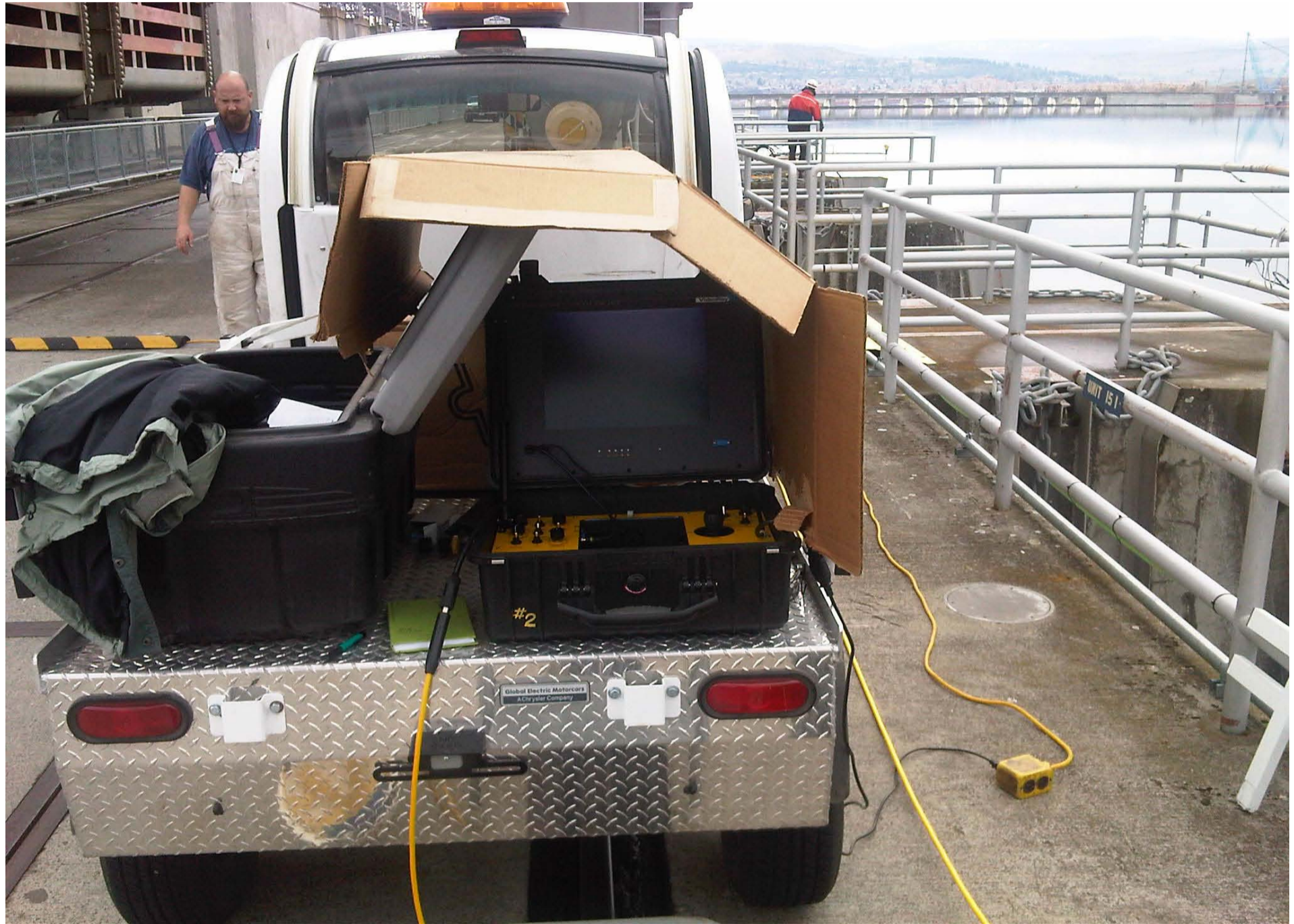
ROV inspection of turbine trashracks for debris accumulation
